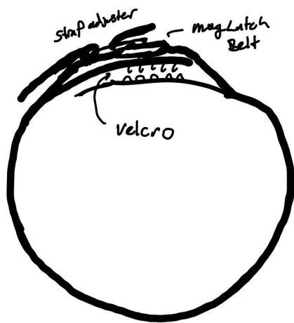
Figure 4: Diagram of Closed Cuff
